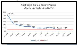
• Several pallets of side rails that were 'on-hold – deemed unweldable' were then welded with the new settings. Results are shown below, 100% passed, all material was recovered.
